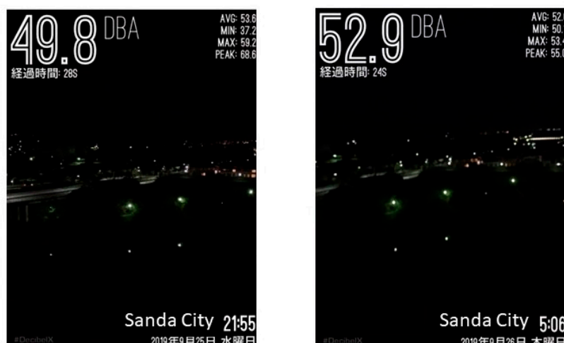
Figure 10. Examples of snapshots from two videos taken at night and in the early morning: Measured values are dB(A), slow peak. The survey was carried out on 25 September 2019.
