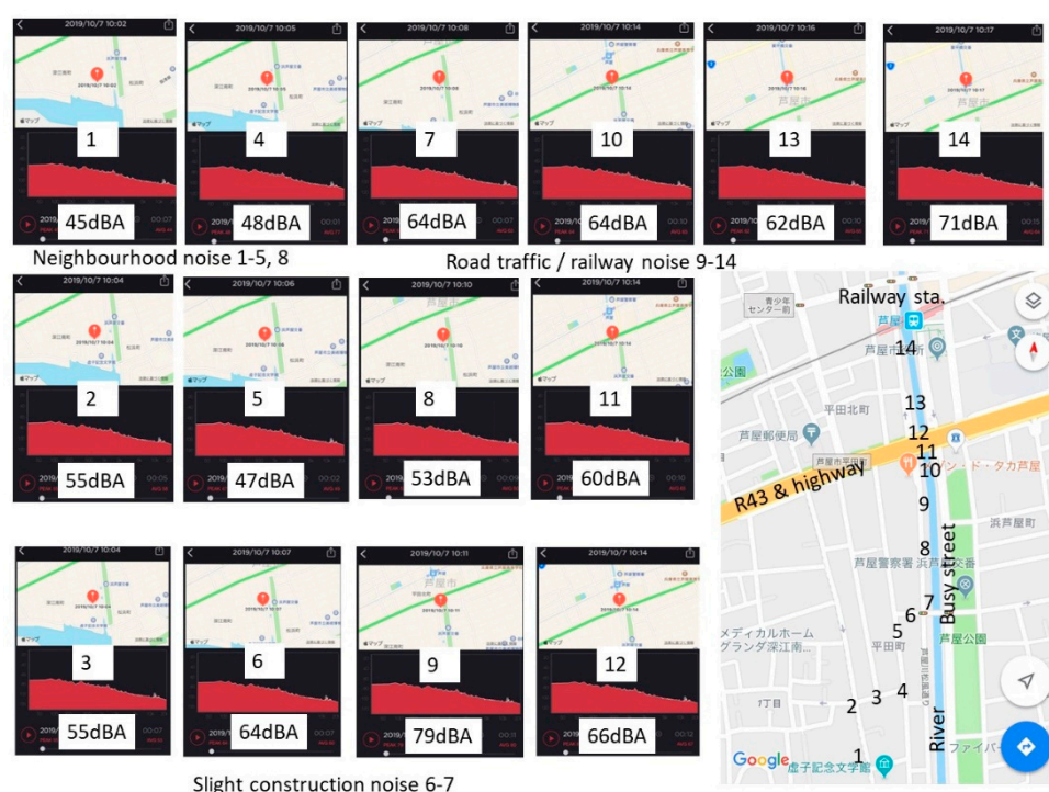
Figure 6. An example of a map with geo-referenced sound data using dB Meter Pro on an iPhone XS: Point 14 is near a railway (Hanshin Railway), and it is at Ashiya Station. Measured values are dB(A), slow peak. The survey was carried out at 10:00–10:20 on 7 October 2019.
