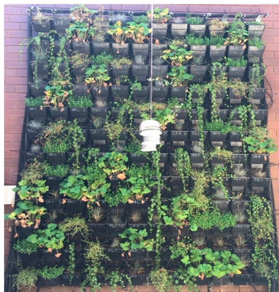
Figure 2. Experimental living wall showing the arrangement of the 144 living wall pots.
