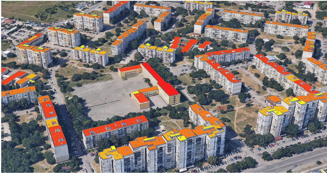
Figure 9. Visualization of classified rooftop areas based on theoretically produced electricity for a one-year period. The Natural breaks classification method is applied, with red indicating the highest energy potential and yellow representing the lowest yield.
