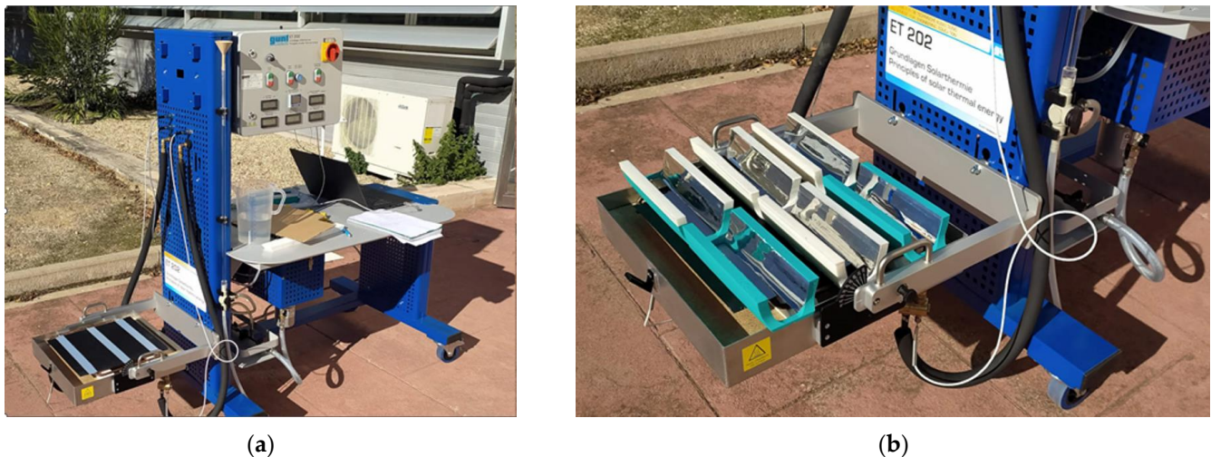
Figure 8. Experimental setup of outdoor experiment using GUNT ET-202 unit: (a) RC film strips adhered to absorber plate, (b) RC film + CPCs positioned above reference aluminum plate.
