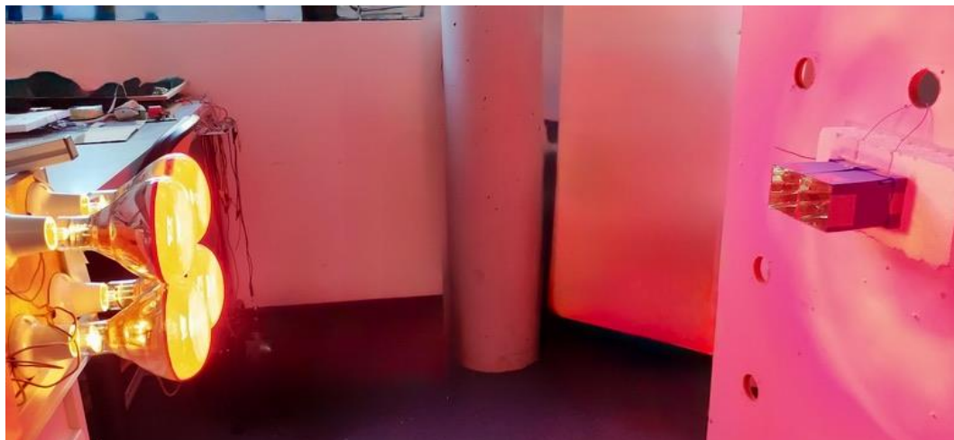
Figure 5. Experimental setup of laboratory test using IR lamp as solar source pointing to two 3D CPC emitters (with and without RC film).
