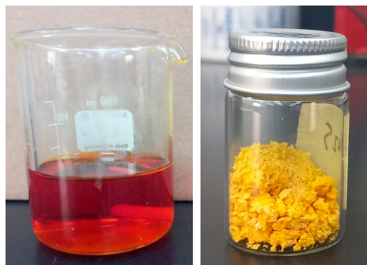
Figure 2. The intermediate solution of \text{Na}_2\text{S} (left) and the dried \text{Na}_2\text{S} at 200 °C under vacuum (right).
