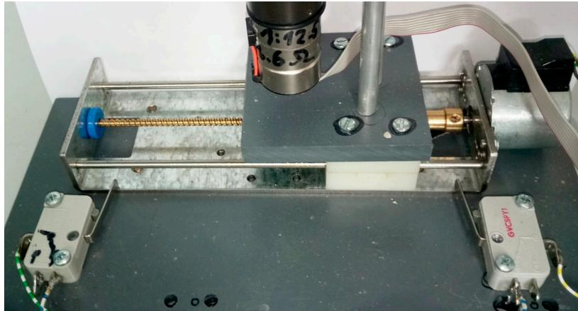
Figure 13. Translation stage with limit switches and mounted motor.
