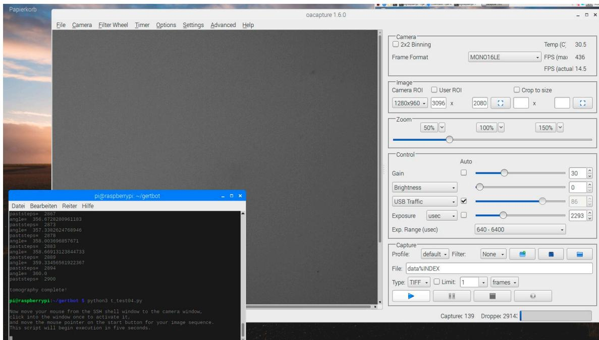
Figure 14. Screen shot of the Astronomy Imaging program oaCapture on the raspberry Pi, with the script window to the left.
