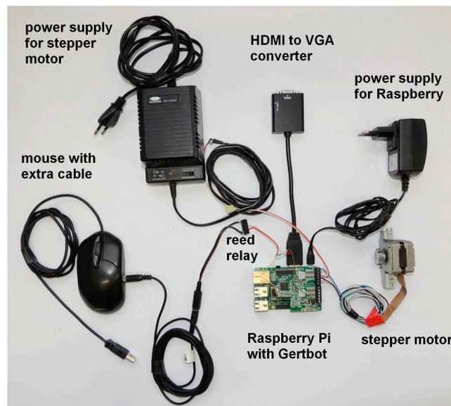
**Figure 10.** Raspberry Pi computer with mounted Gertbot board, the modified computer mouse and a connected stepper motor.
