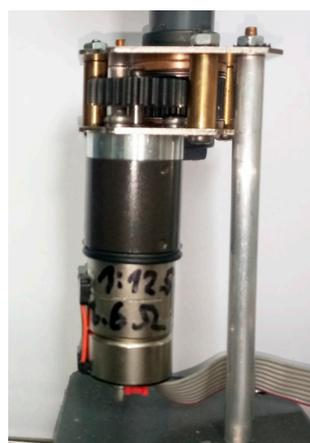
**Figure 12.** Stepper motor with reduction gear.
