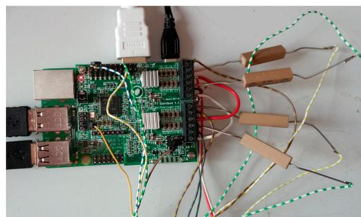
**Figure 11.** Shows the Pi and Gertbot with additional power resistors to match the required current for the stepper motors.
