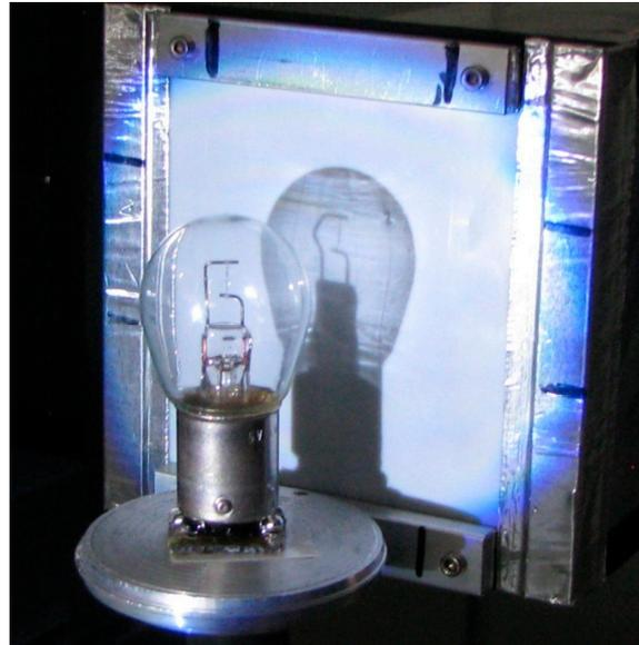
**Figure 15.** Optical projection of a light bulb onto a matte screen in the detector box.
