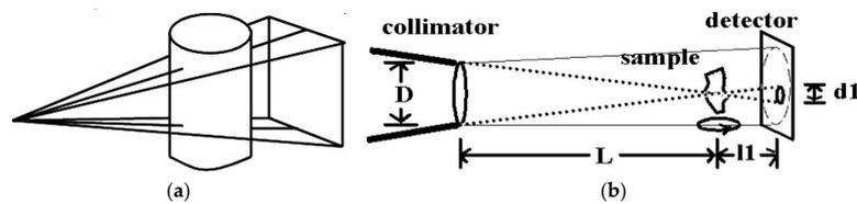
**Figure 1.** (a) This is a figure magnifying cone beam projection, (b) beam geometry for neutron imaging: Approximation to parallel beam.
