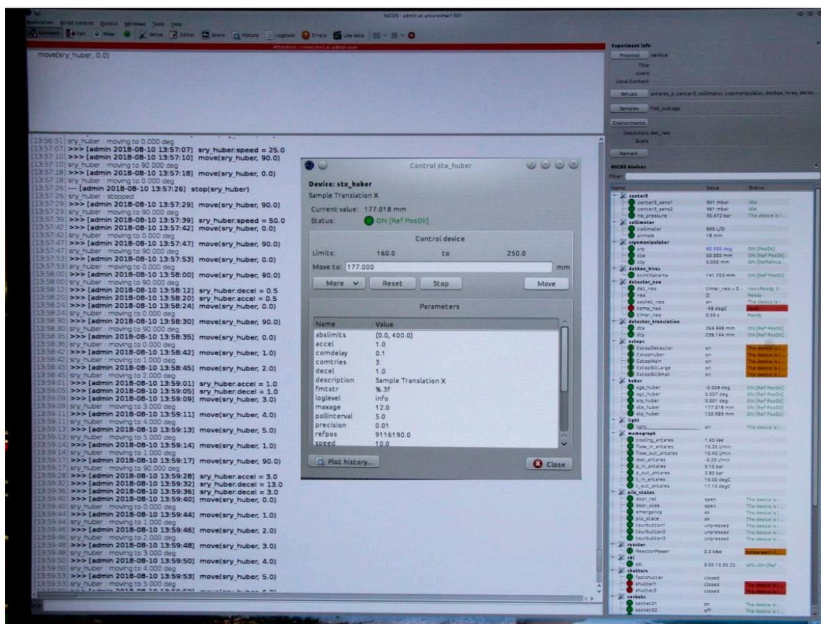
**Figure 8.** Screenshot of NICOS control software with history, command line, a control widget for a motor axis, and the device list.
