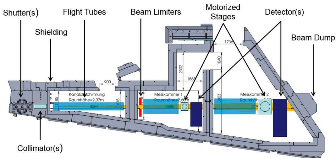
**Figure 2.** The ANTARES neutron imaging facility at the FRM II reactor, with the reactor to the left, and two measurement chambers. The irregular shape is given by external walls and other neighboring instruments.
