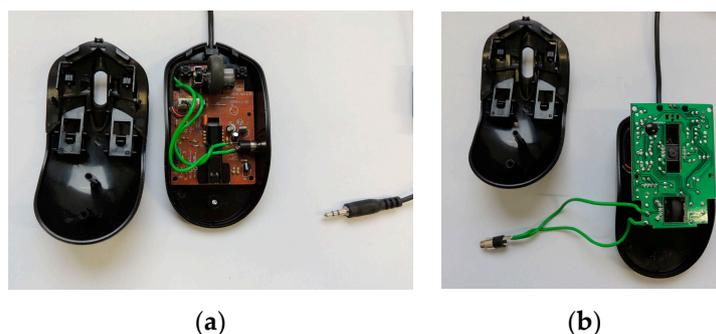
**Figure 9.** Modified computer mouse with extra connection to the left mouse button – extra socket built in (a) and simple soldered connection to the button (b).
