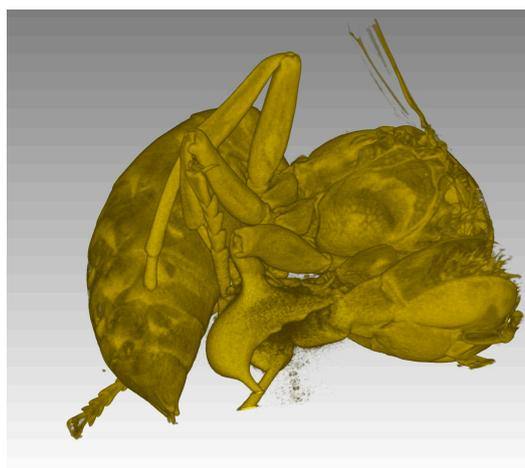
**Figure 7.** Neutron CT with 9  $\mu\text{m}$  voxel size.
