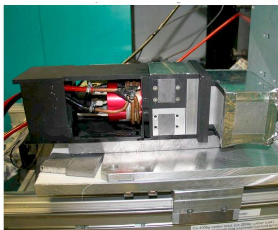
**Figure 4.** Detector with water cooler.
