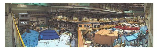
**Figure 1.** Artistic panoramic view into an experimental hall of the Materials and Life Science Facility at J-PARC [2–5]. The neutron beam ports surrounding the target station are to the far right feeding beamlinces at the right, while muon apparatus is located in the left side of the image.
