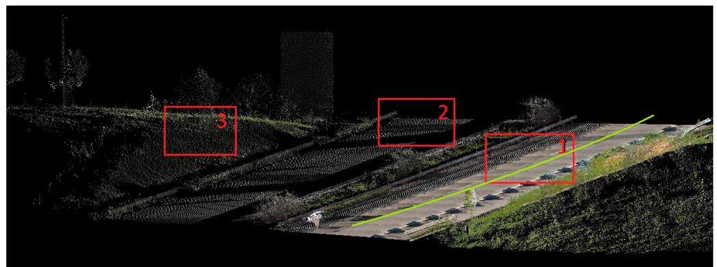
**Figure 2.** An MLS point cloud sample of an actual road being surveyed. Rectangles 1, 2, and 3 contain, respectively, 25,000, a few tens, and approximately 500 points.
