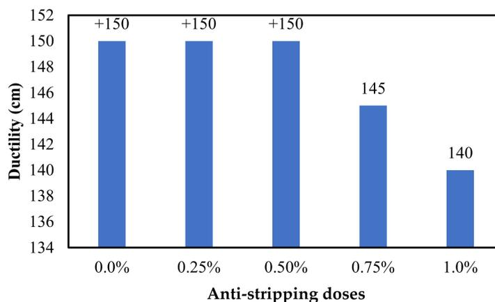
**Figure 4.** Ductility results of asphalt binder.
