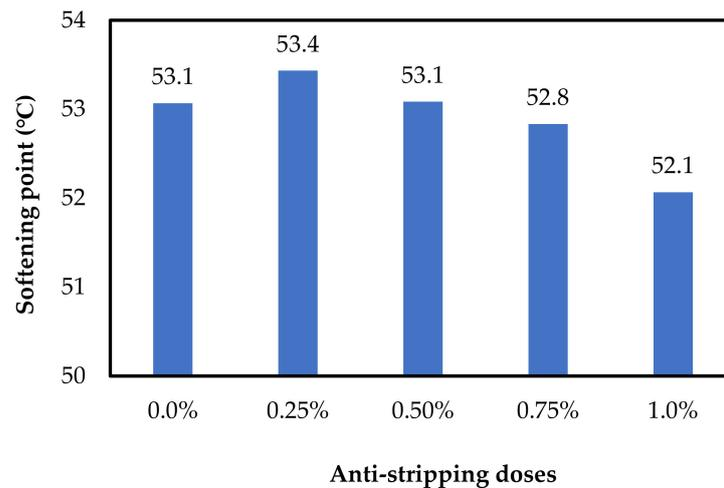
Figure 3. Softening point of asphalt binder.
