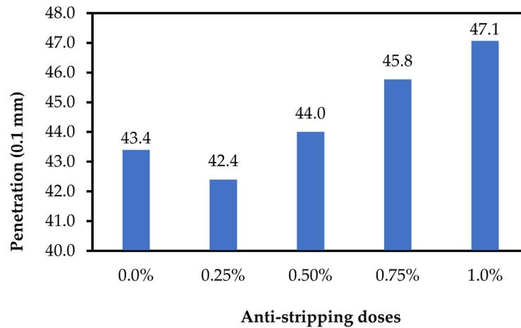
Figure 2. Penetration results of asphalt binders.
