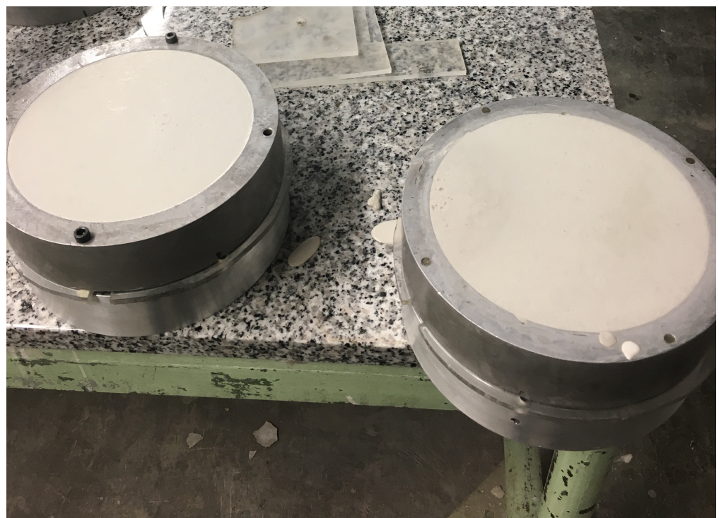
Figure 6. Cast specimens in rings measuring 21.6 cm in diameter and 5.1 cm tall for the small direct shear machine. Note the plexiglass rings measuring 0.3 cm thick isolating the lift line from hydrostone penetration during casting.
