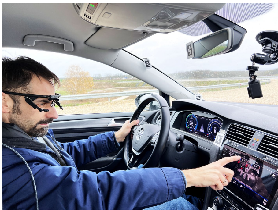
Figure 2. Test apparatus: Pupil Core eye-tracking device installed on the head of driver; HD camera in front of the driver; ID tags in the view of driver (around windshield and center console).
