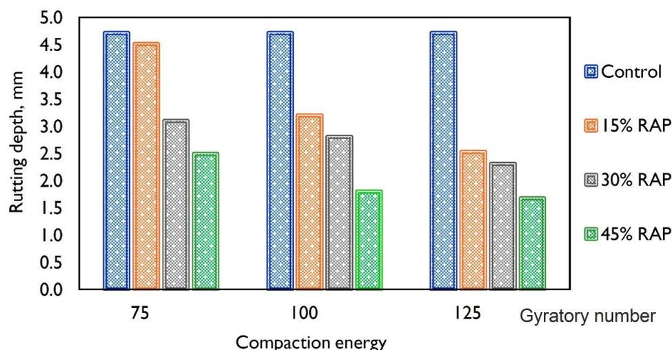
Figure 6. Results of the permanent deformation tests (HMA without additives).
