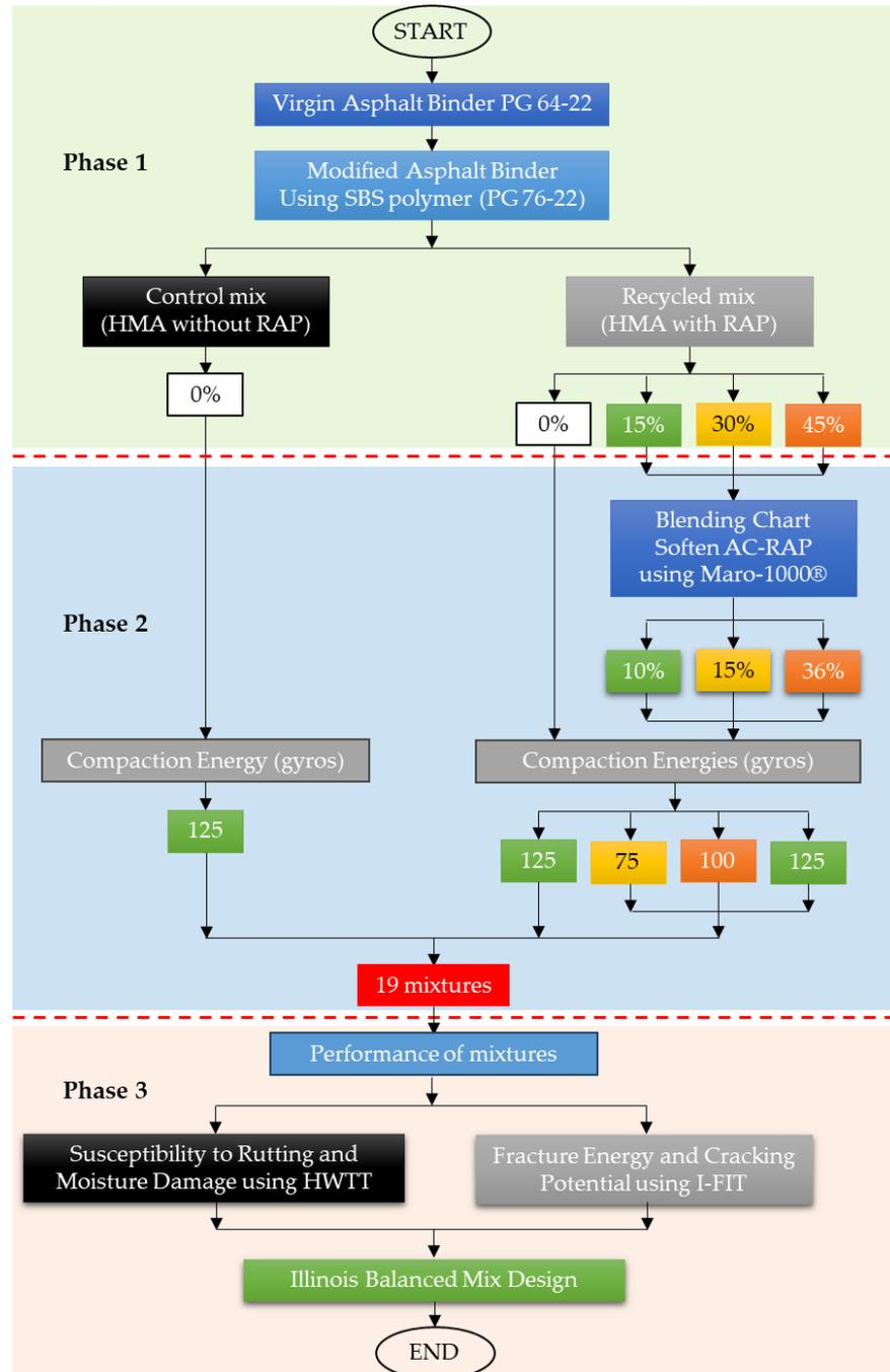
Figure 1. Flow chart of the experimental design.
