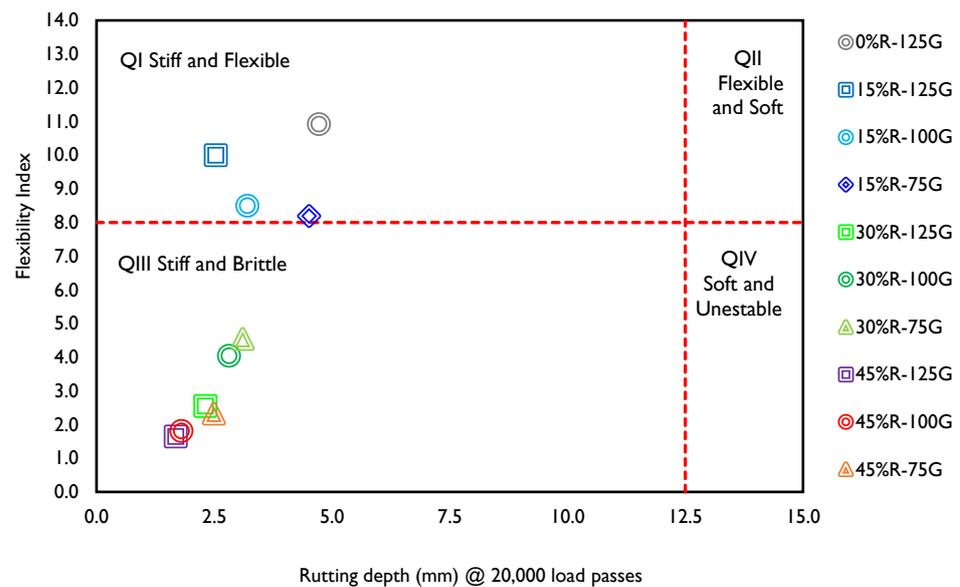
**Figure 10.** Performance interaction diagram for HMA without the rejuvenating additive—relationship between RD and FI.
