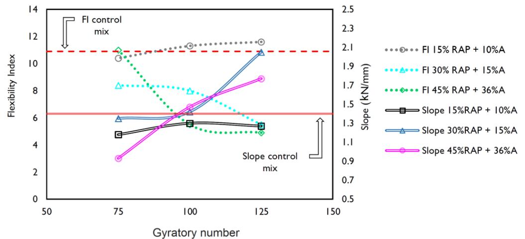
**Figure 9.** Results of the flexibility index test (I-FIT) for the recycled HMA with a rejuvenating additive.
