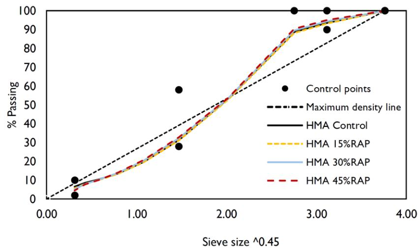
Figure 4. Designed aggregate gradation aligned with the control points for a 1/2" nominal size diameter HMA.
