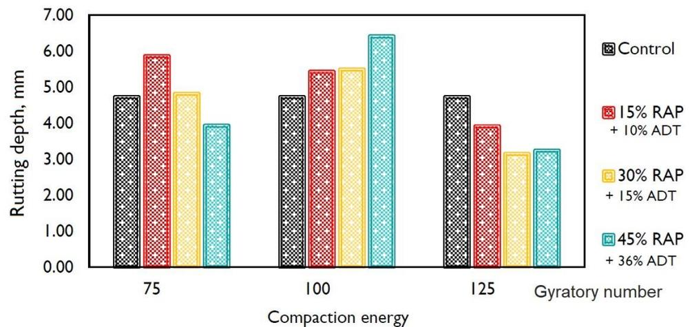
Figure 7. Results of the permanent deformation test (HMA with additive).
