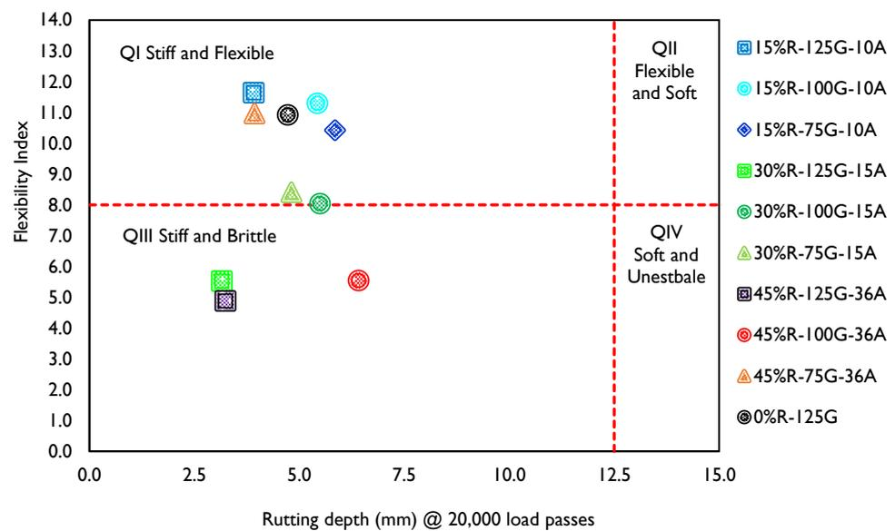
Figure 11. Performance interaction diagram of RD and FI for HMA with a rejuvenating additive.
