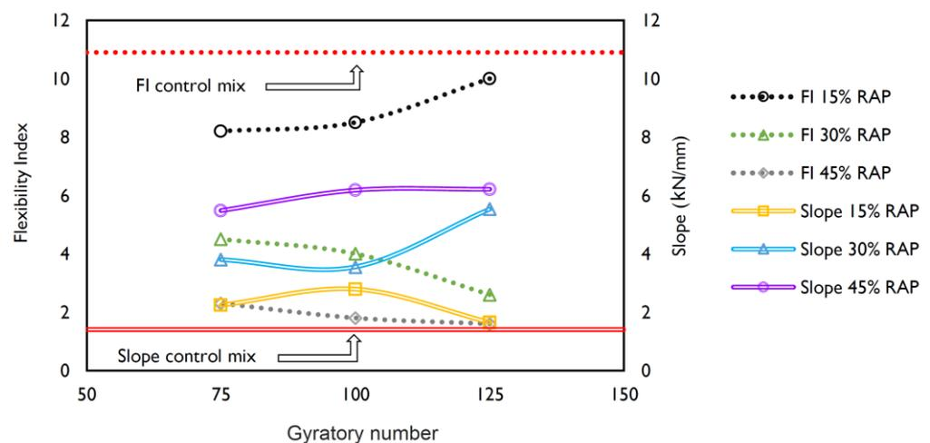
**Figure 8.** Results of the flexibility index test (I-FIT) for recycled HMA without additive.
