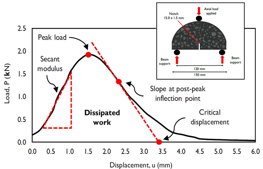
**Figure 5.** Typical representation of the flexibility index in the semi-circular load–displacement curve.
