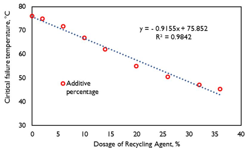
**Figure 3.** Determination of the additive content.
