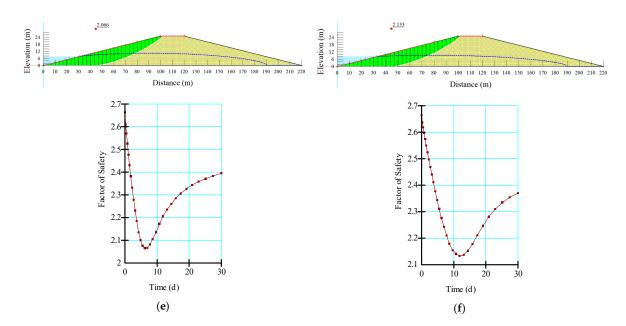
**Figure 5.** Trends in the factor of safety values for (a) 1:1 (V:H) without toe drain and instantaneous drawdown (b) 1:1 (V:H) without toe drain and 10-day drawdown (c) 1:1 (V:H) without toe drain and 1 m per day drawdown (d) 1:4 (V:H) with 30 m toe drain and instantaneous drawdown (e) 1:4 (V:H) with 30 m toe drain and 1 m per day drawdown.
