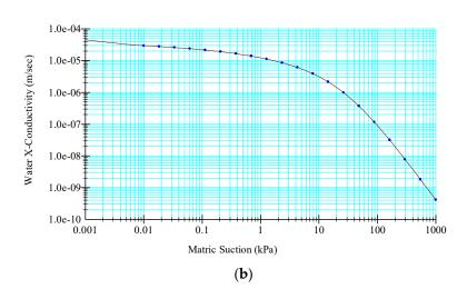
Figure 2. Functions of (a) volumetric water content, and (b) hydraulic conductivity.
