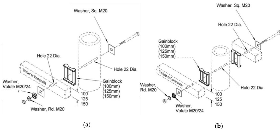
Figure 4. Predrilled crossarm assembly: (a) single crossarm; (b) double crossarm [31].
