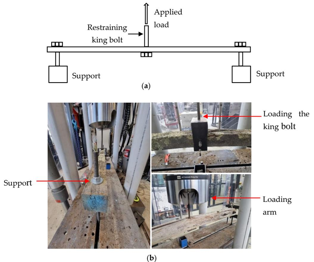
Figure 5. Three-point bending test setup: (a) schematic representation; (b) actual test setup.
