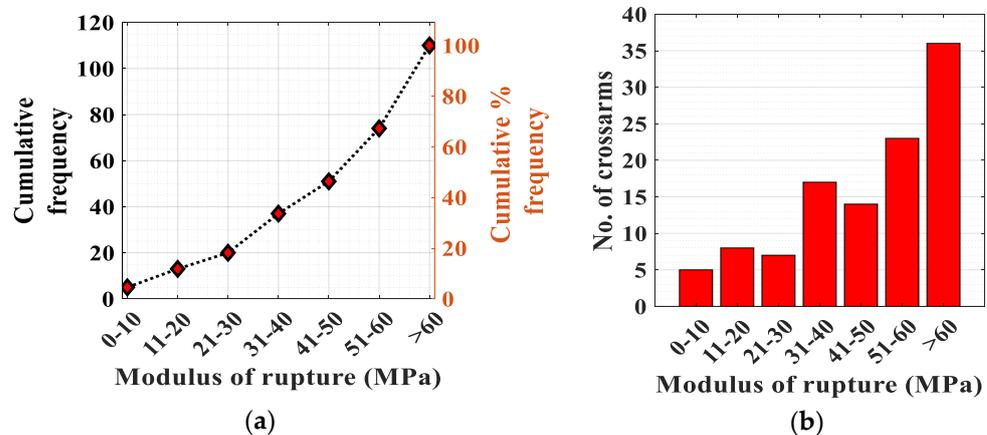
Figure 6. (a) Variation of the modulus of rupture—110 specimens; (b) groupings of the modulus of rupture.
