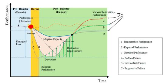
Figure 1. Performance based resilience components of a CIS (adapted from Refs. [28,48]).
