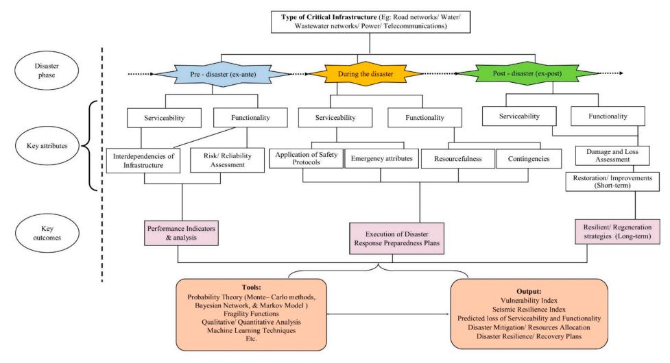
Figure 12. An overview of an integrated and adaptive framework for assessing infrastructure resilience for earthquake hazards.
