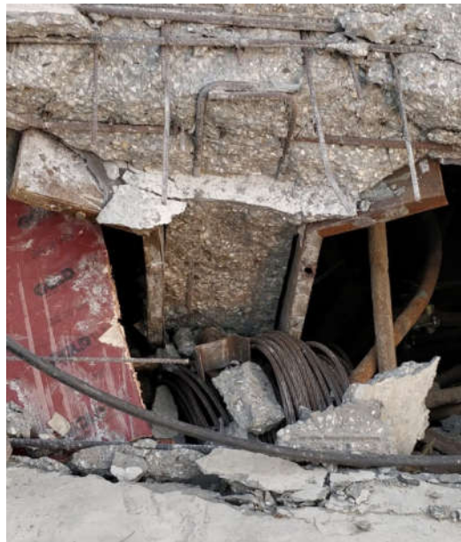
Figure 8. L-bar of fractured beam, anchorage failure of some slab rebar, bearing failure of formwork around bolting holes, and prestressing cables pulled out to significant length and bent.
