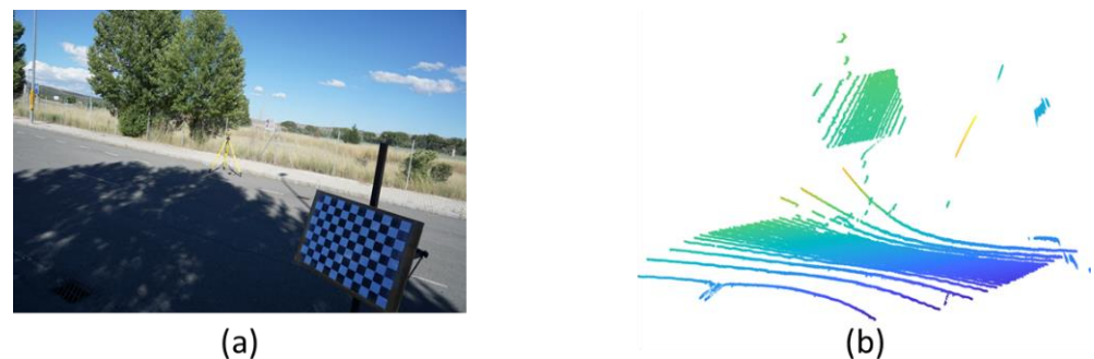
Figure 7. Calibration between the LiDAR sensor and the camera. (a) image acquired of the checkboard. (b) point cloud acquired of the checkboard.
