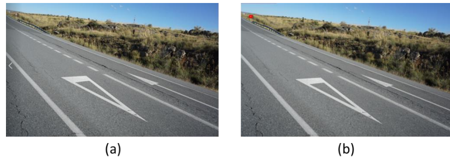
Figure 11. Example of an extreme situation where (a) Traffic sign is omitted by the manual labeller. (b) Traffic sign is detected by the deep learning architecture.
