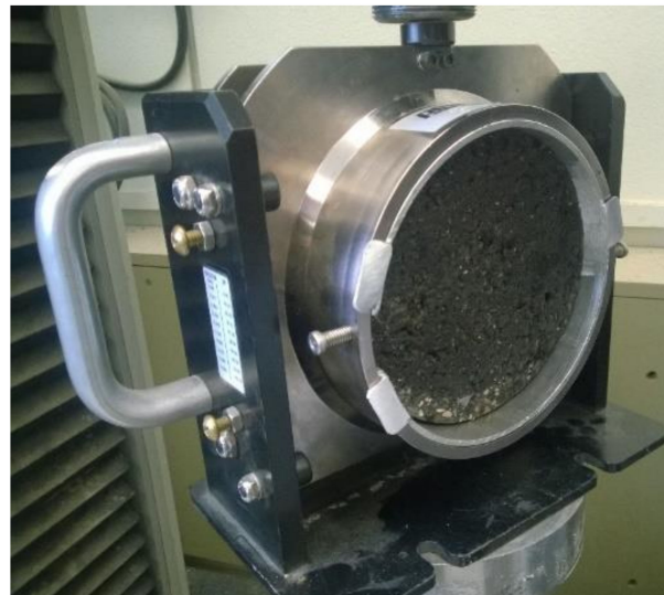
Figure 3. Test apparatus of interface shear test.
