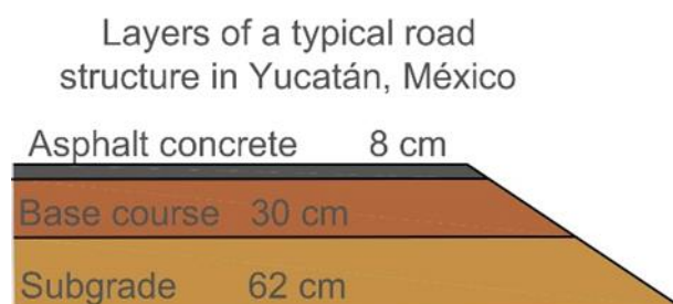
Figure 2. Schemes of layers and thickness of a typical road structure in Yucatán [23].
