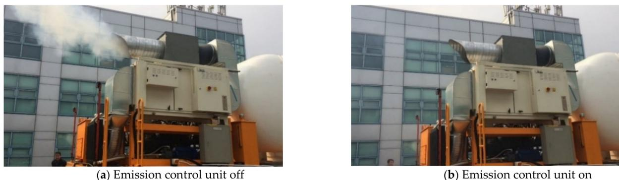
**Figure 2.** Heating equipment with the emission hood unit.
