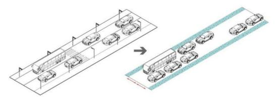
**Figure 7.** Supposed more efficient utilisation of the carriageway given by the development of CAVs [48].
