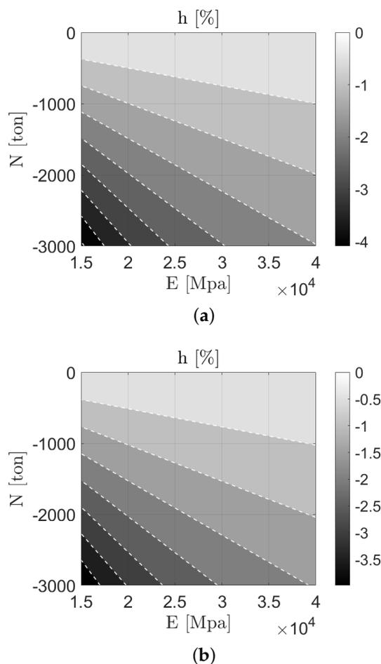
**Figure 4.** Percentage variation of the natural frequency in externally prestressed beams expressed by the  $h$  ratio in Equation (10), given two sample cases (a) with  $A = 6 \text{ m}^2, I = 4 \text{ m}^4, \nu = 0.2, \rho = 2500 \text{ kg/m}^3$  and (b) with  $A = 2 \text{ m}^2, I = 4 \text{ m}^4, \nu = 0.2, \rho = 2500 \text{ kg/m}^3$ .
