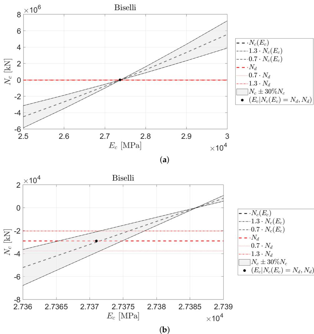
**Figure 5.** Estimated values of the elastic modulus to yield the design prestressing value within the given  $\pm 30\%$  confidence bounds: (a) spans between 25,000 and 30,000 MPa, (b) focuses on the estimated value.
