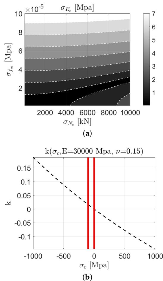
**Figure 3.** Percentage variation of the natural frequency expressed by the approximate  $k$  ratio in Equation (7). (a) The variation of both  $E$  and  $\sigma_c$ ; (b) the dependence of the  $k$  factor on the natural sole compression stress given the elastic modulus. The solid vertical lines in (b) indicate the range of interest in existing concrete structures, averaging between  $-100$  and  $0$  MPa.
