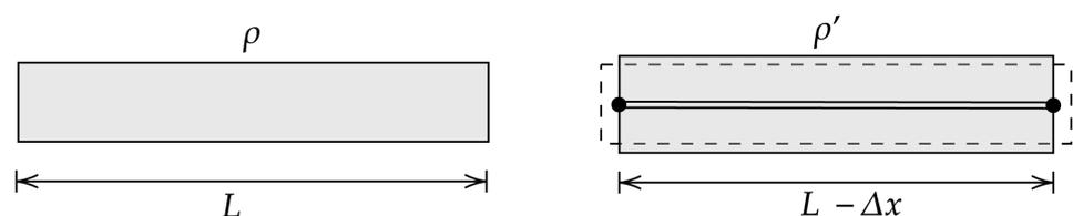
Figure 2. Effect of axial compression in volume contraction.
