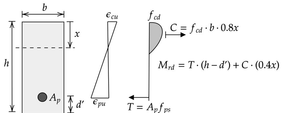
**Figure 1.** Evaluation of the resisting bending moment of a prestressed beam, where  $\epsilon_{cu}$  and  $\epsilon_{pu}$  are the ultimate deformations of concrete and the prestressing cable,  $f_{cd}$  is the design concrete stress and  $f_{ps}$  is the design tensile stress of the prestressing cable,  $M_{rd}$  is the resisting design moment.
