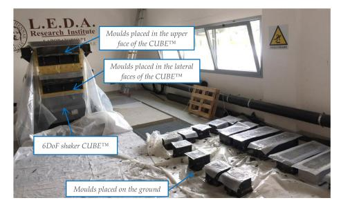
Figure 3. Experimental set-up for evaluating the influence of vehicle-induced vibrations.
