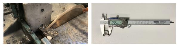
(a) Diamond blade saw(b) Sample measurementFigure 2. Scanning electron microscope sample preparation for microscopic observation.
