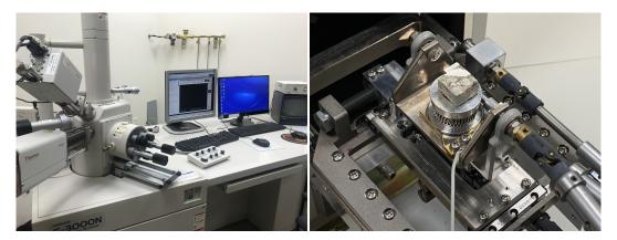
(a) Hitachi 3000N SEM Microscope(b) Sample inside SEM MicroscopeFigure 1. Scanning electron microscope and sample mount for microscopic observation.
