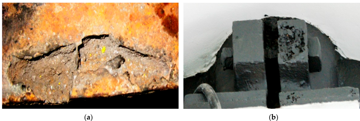
Figure 17. Casting defects of the cast-iron girders: (a) gas blowhole, (b) slag inclusion.
