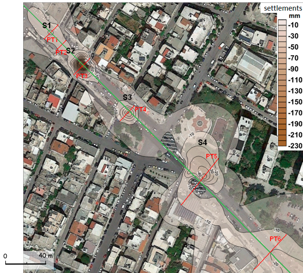
Figure 7. Settlement contours during the excavation of the Athens Metro Line 2 in the Panagi Tsaldari Avenue area superimposed on Google Map background. High subsidence contours are shown by increased color grading. White dashes indicate areas in which monitoring benchmarks were destroyed and replaced, and observations were discarded because they record only part of the ground deformation. Asymmetries in the subsidence trough (ground loss) related to the distribution of buildings and greenfield areas suggest that observations on buildings underestimate subsidence due to sSSI. For significant results, only settlements above 10 mm are examined in this article.
