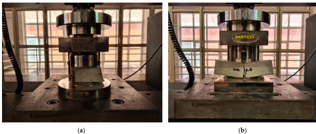
Figure 3. Test setup: (a) compression and (b) flexural test on the matrix.
