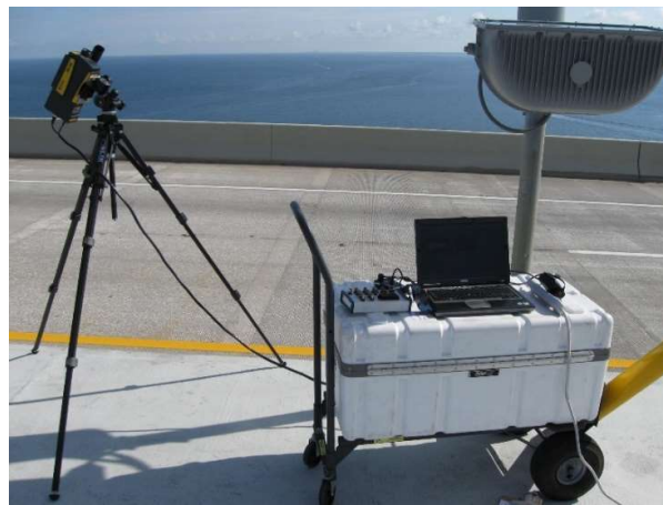
Figure 2. The Laser vibrometer used in the field measurement.
