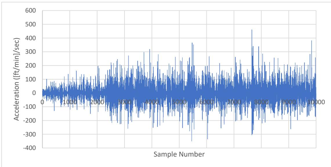
**Figure 12.** Plot of acceleration ((ft/min)/sec) versus sample number on 23 July, 2015. The sum of the acceleration over 9999 readings was 323 (ft/min)/sec.
