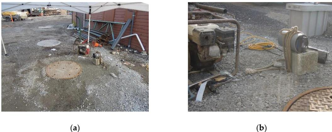
**Figure 1.** Near surface air velocity and temperature. (a) The general area of the study. (b) The probe of the thermoanemometer is visible in the picture. The probe is approximately 20 cm above the ground and oriented approximately north–south in the horizontal plane. This height and the canopy above provided protection to the probe from dust and rain.
