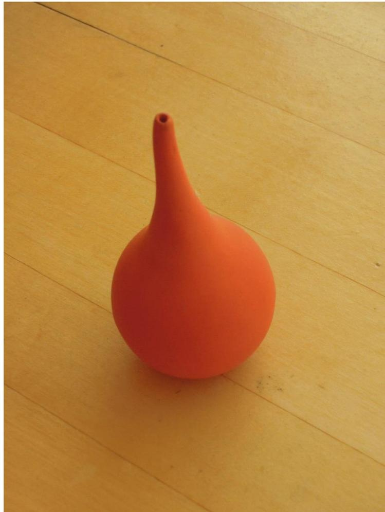
**Figure 14.** Helmholtz resonator. This ear syringe has the same shape as the resonators designed by Helmholtz. Classic Helmholtz resonators have a single opening to the atmosphere, a hollow neck and an enclosed airspace.
