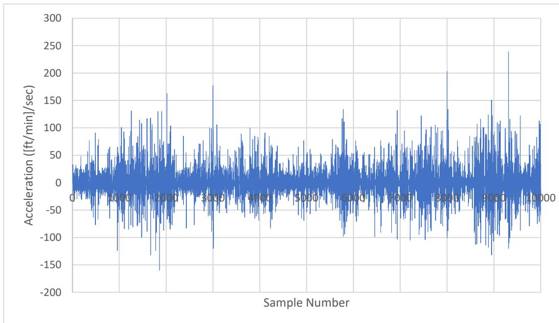
**Figure 11.** Plot of acceleration ([ft/min]/sec) versus sample number on 10 March, 2015. The sum of the acceleration over 9999 readings was 142 (ft/min)/sec.
