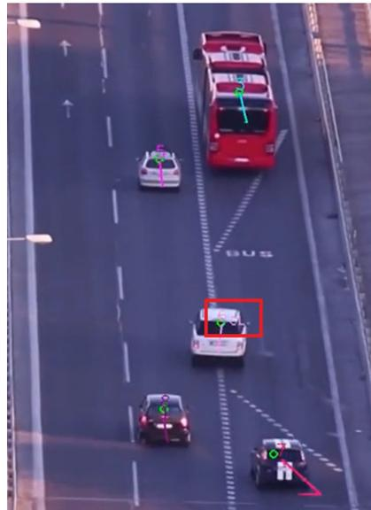
Figure 6. Example of detection result (solid-line-crossing behavior).
