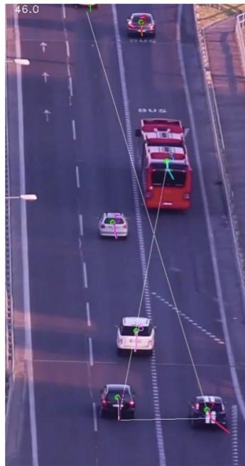
**Figure 8.** Tracking errors caused by the Hungarian algorithm (white lines) can be corrected by a Kalman filter (colored lines).
