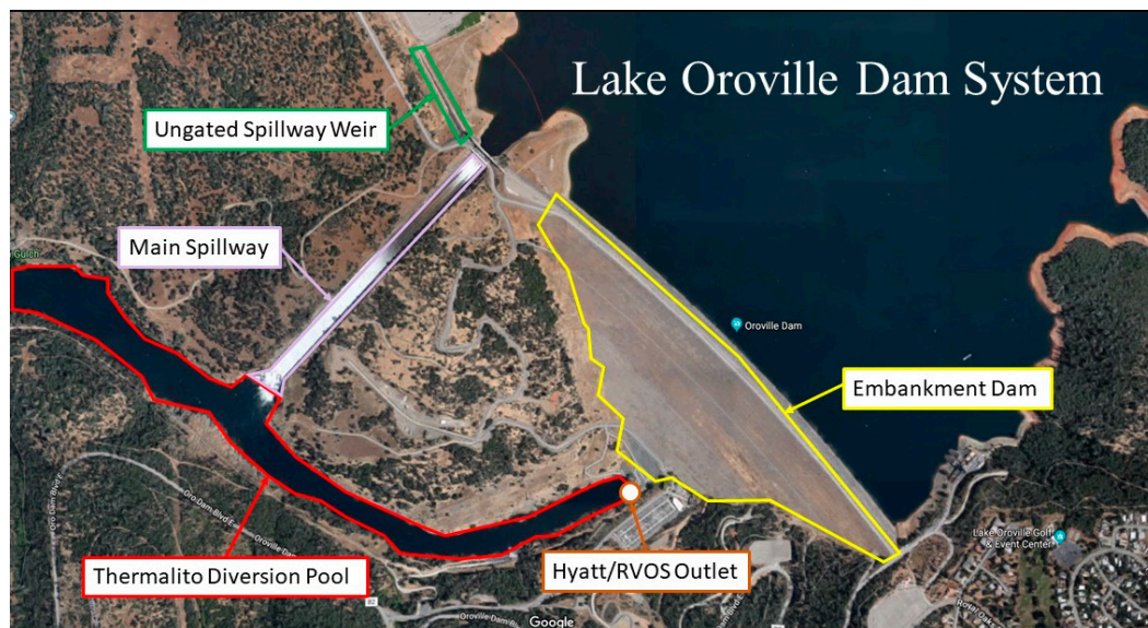
Figure 1. Lake Oroville Reservoir is enclosed to the south east by a 770-foot-tall earth-fill embankment dam, which is the tallest dam in the United States. All mechanisms for water removal drain to a diversion pool that has a lower elevation. The Hyatt Powerhouse and RVOS discharge into the upstream end of the common diversion pool, followed by the main spillway, and the approximate path of the ungated spillway, which drains furthest downstream. Water flows from the diversion pool through other structures regulating the flow of the Feather River.
