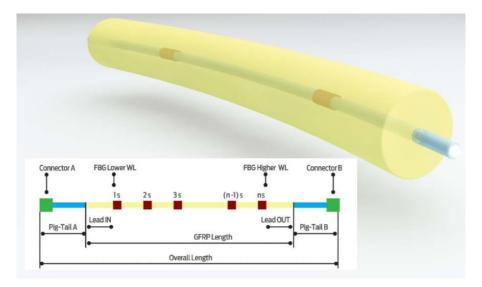
Figure 1. Fiber Bragg grating (FBG) configuration with Draw Tower Gratings (DTG<sup>®</sup>) [15].
