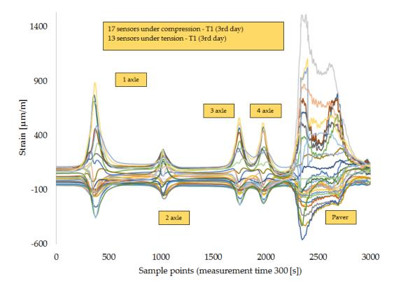
**Figure 14.** Monitoring of T1 on the third day of the paving process when the four-axle truck and the paver drove along the FBG chain of 30 DTG<sup>®</sup> (L1) embedded under the first base asphalt layer (AC-14) [17].
