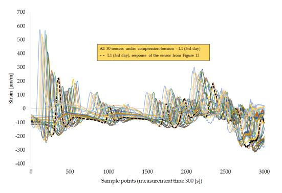
**Figure 15.** Monitoring of L1 on the third day of the paving process when the four-axle truck and the paver drove along the FBG chain of 30 DTG<sup>®</sup> (L1) embedded under the first base asphalt layer (AC-14).
