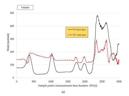
**Figure 11.** Strain values of sensors: (a) T1' and T1", (b) T2' and T2" at a temperature of 21 °C, and (c) T3' and T3" at a temperature between 24 and 29 °C during the construction of the CyPaTs asphalt pavement on the third day.
