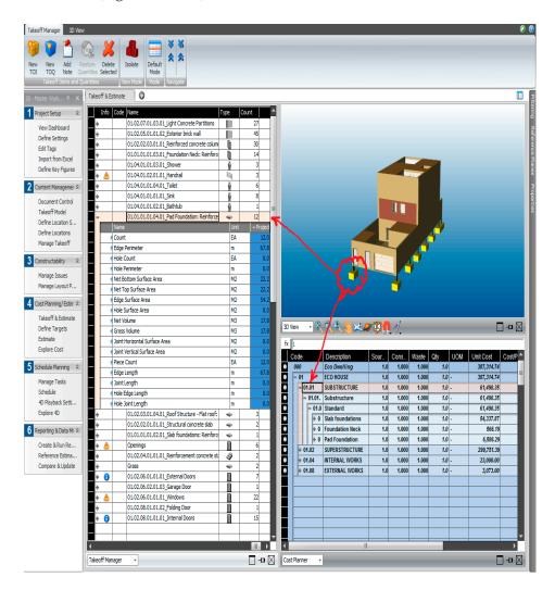
Figure 8. Take-off and cost estimation integrated with the 3D Model.
