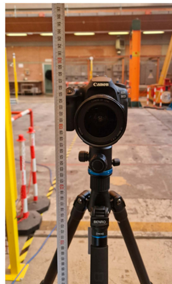
Figure 4. Verification of the camera height (131 cm) above the floor, matching the height of the monitored target, measured with a graduated staff placed in front of the lens.
