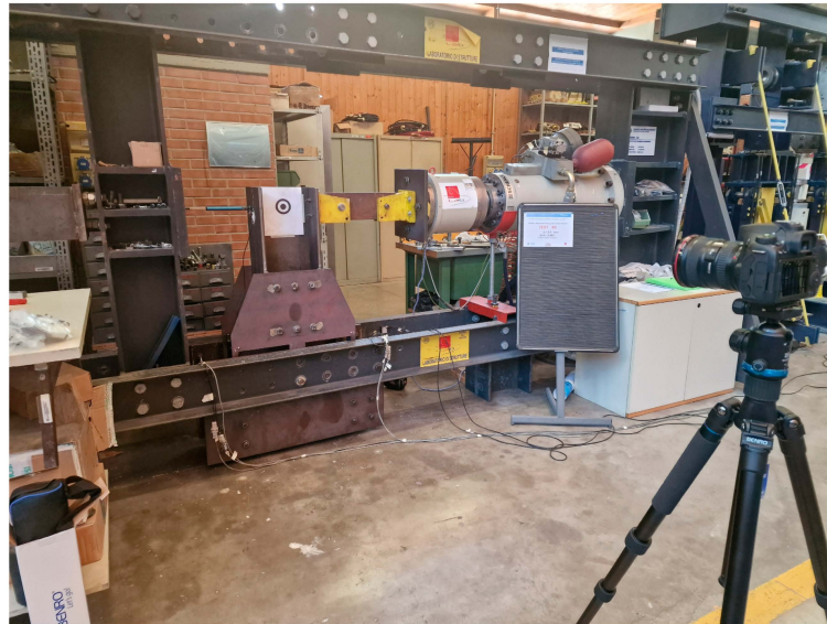
Figure 3. Laboratory test setup: digital camera positioned frontally with respect to the instrumented portal-frame specimen, at a fixed distance and height from the monitored target.
