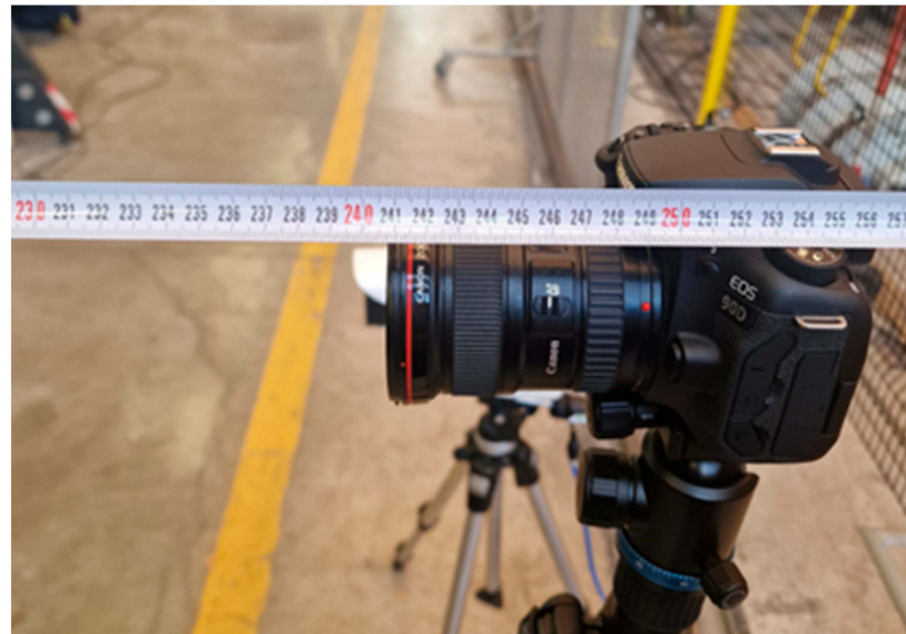
Figure 5. Verification of the camera-to-target longitudinal distance (240 cm), measured with a tape stretched in front of the lens.
