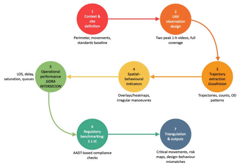
Figure 8. Integrated workflow for Vision Zero-oriented risk diagnosis combining UAV-based trajectory analysis (GoodVision), operational performance modelling (SIDRA INTERSECCION) and regulatory benchmarking (Norma 3.1-IC), supplemented by descriptive crash context.
