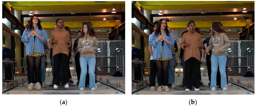
Figure 15. During (a) and immediately after (b) the 16 people jump with a_{pic} = 3.4 \text{ m/s}^2 .
