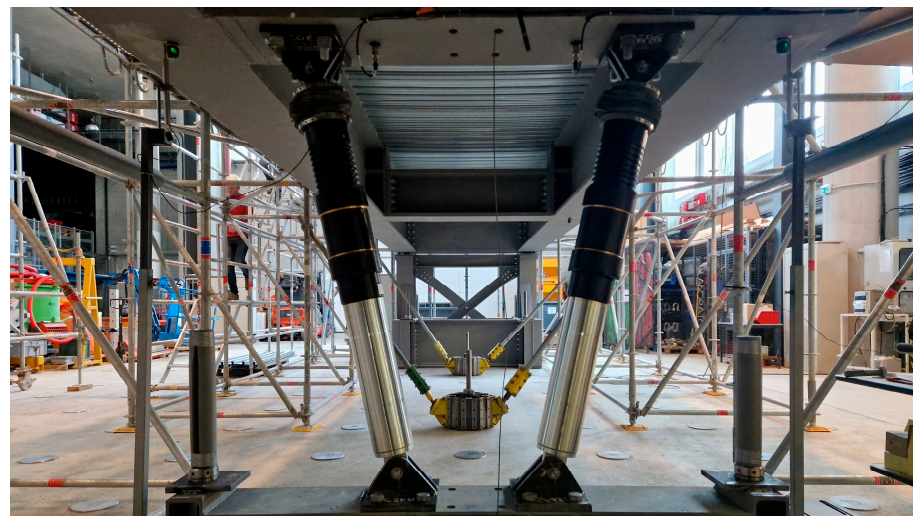
Figure 3. Removable pair of viscous dampers.
