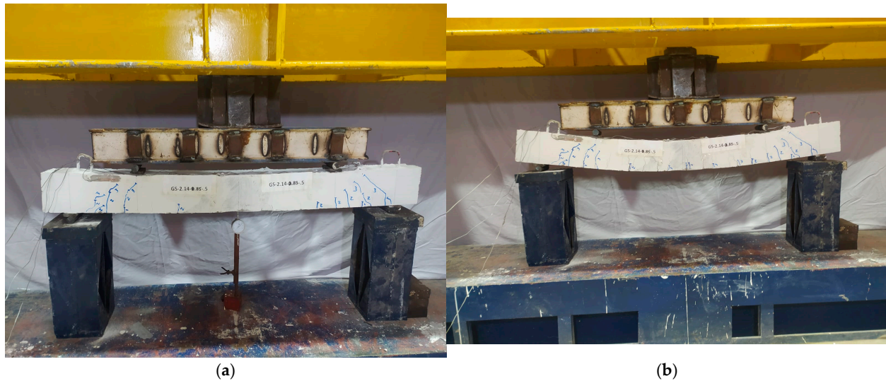
Figure 11. Deflection of beam GS-2.14-.85: (a) measured at ultimate load, and (b) measured at far post-peak load.
