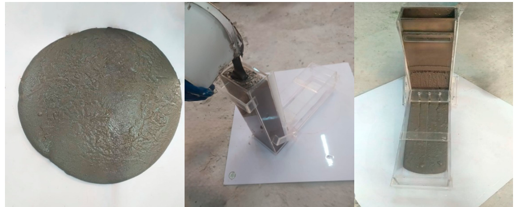
Figure 2. Slump-flow and L-box tests.
