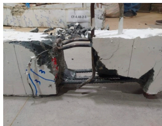
Figure 9. The dowel action for GS-2.14-2.
