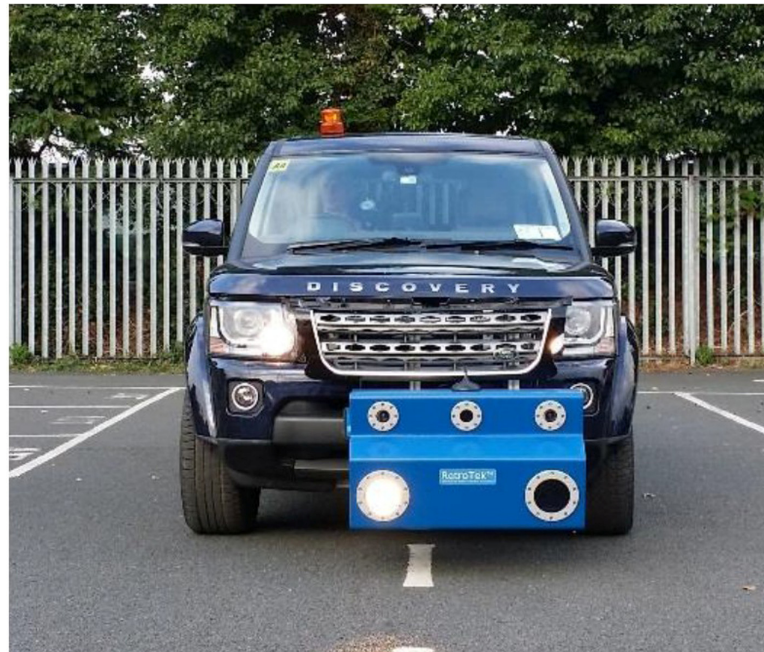
Figure 1. Depiction of a RetroTek-M device installed on the front of a vehicle.
