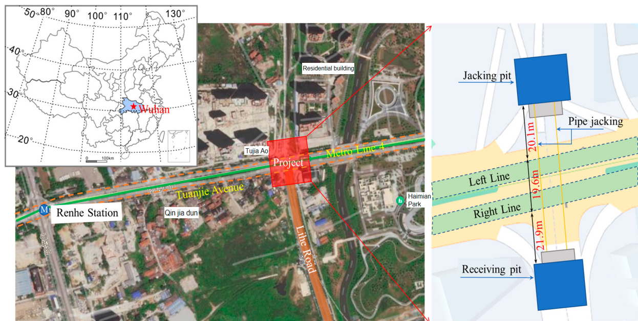
Figure 1. Geographical location of the utility tunnel and its spatial relationship with the shield tunnel.
