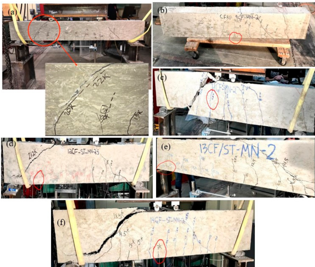
Figure 13. Mode of failure for beam (a) 3CONT_MN_2, (b) CF_MN_2, (c) GF_MN_2, (d) CF_ST_MN_2.5, (e) CF_ST_MN_2, and (f) GF_ST_MN_2.
