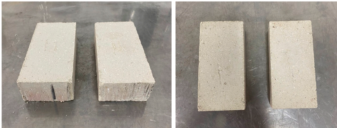
Figure 3. Hyperpressed brick specimens molded under a compaction pressure of 28 MPa.
