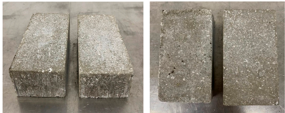
Figure 11. Hyperpressed brick specimens produced with gray Portland cement and molded under a compaction pressure of 41 MPa.
