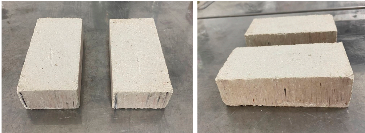
Figure 8. Hyperpressed brick specimens molded under a compaction pressure of 41 MPa.
