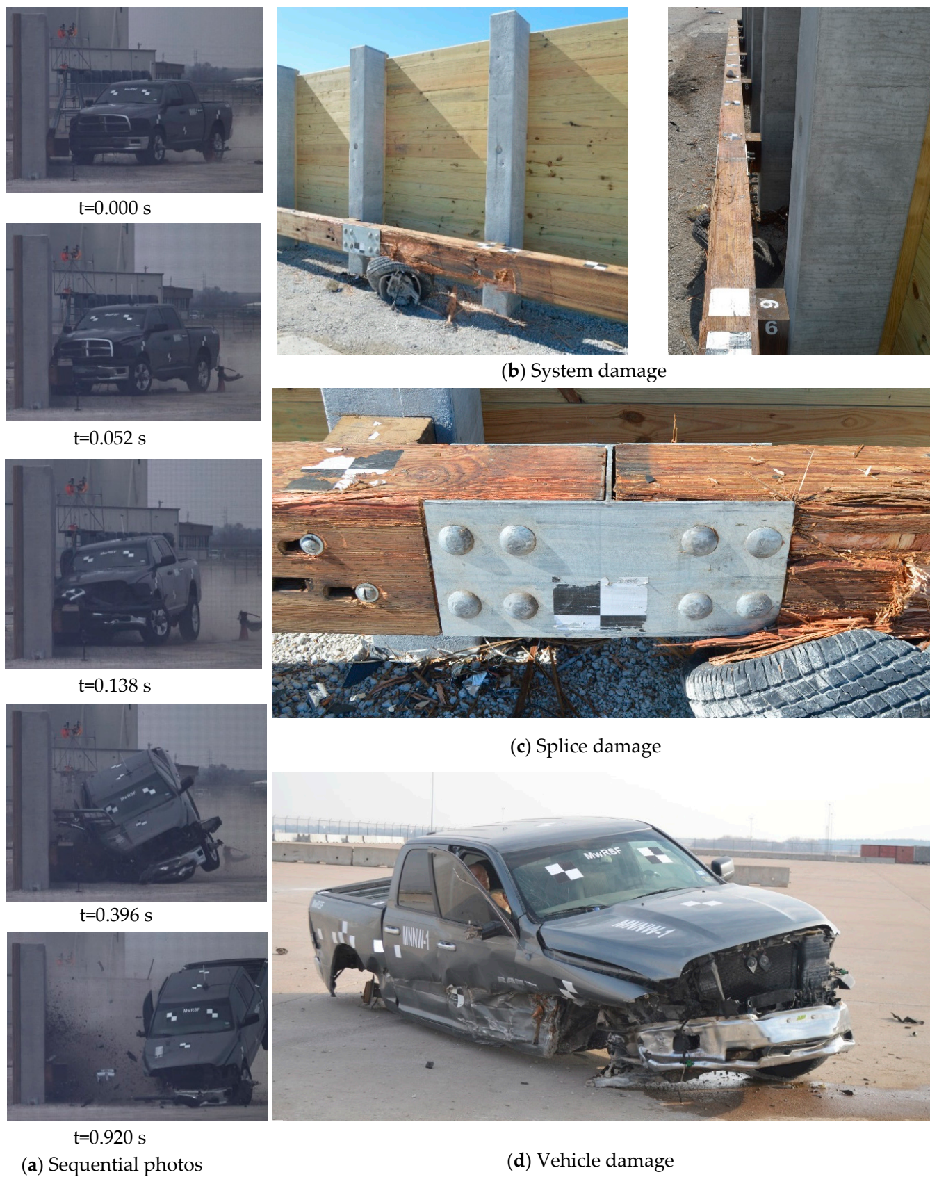
Figure 6. Results from test MNNW-1: (a) sequential crash test photos, (b) overall system damage, (c) splice damage, and (d) vehicle damage.
