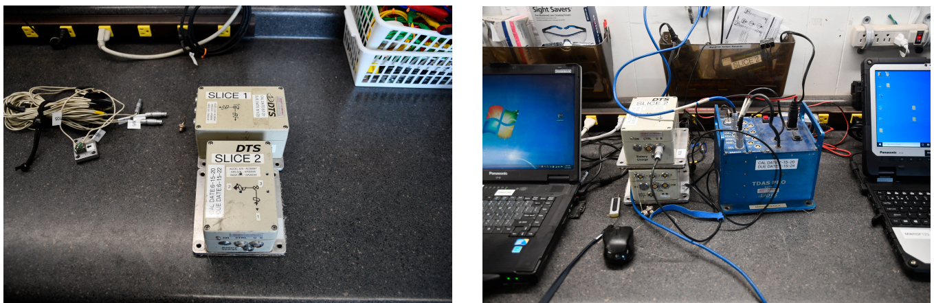
Figure 5. Photograph of SLICE-1 and SLICE-2 accelerometer packages.
