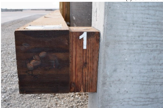
(d) Rubrail, offset blocks, and rail splice (test MNNW-3)
