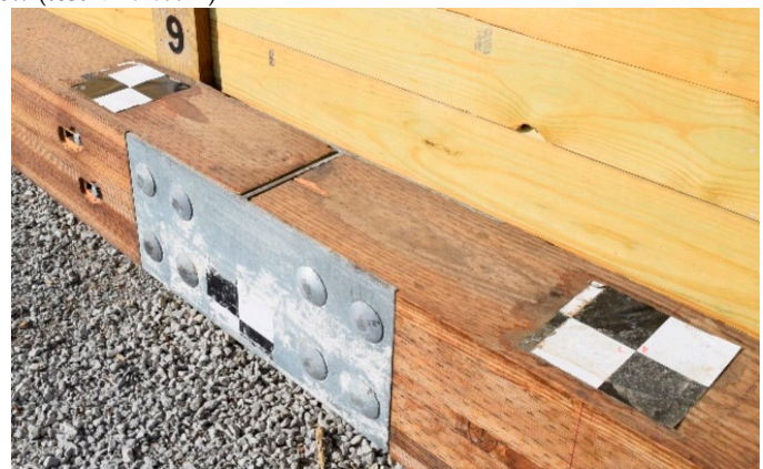
(d) Rubrail, offset blocks, and rail splice (test MNNW-3)
