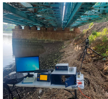
Figure 3. Laser Doppler Vibrometer (LDV) setup to record vertical displacement of bridge during train passage.
