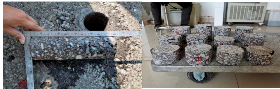
Figure 6. Field coring and laboratory testing of asphalt samples.
