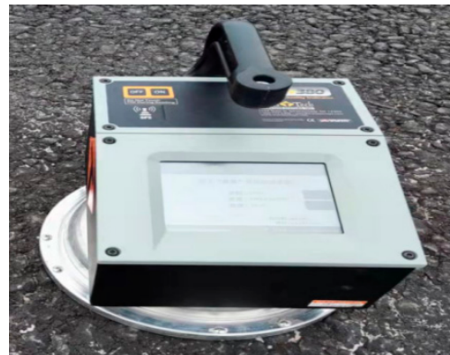
Figure 2. PQI380 type coreless densitometer measurement.
