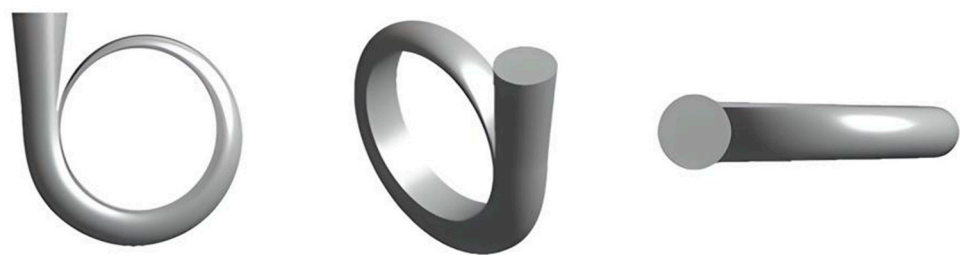
Figure 3. Three-dimensional model of the pump volute.
