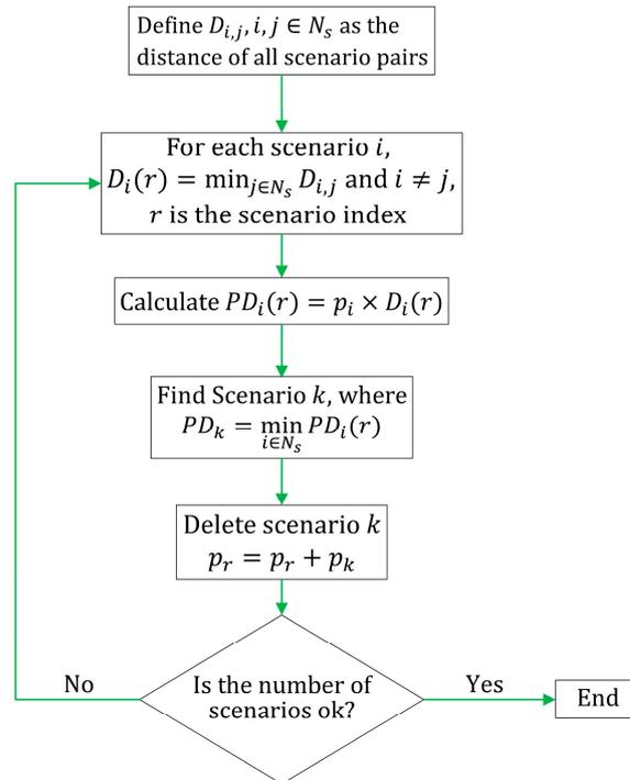
Figure 12. Simultaneous backward scenario reduction method.
