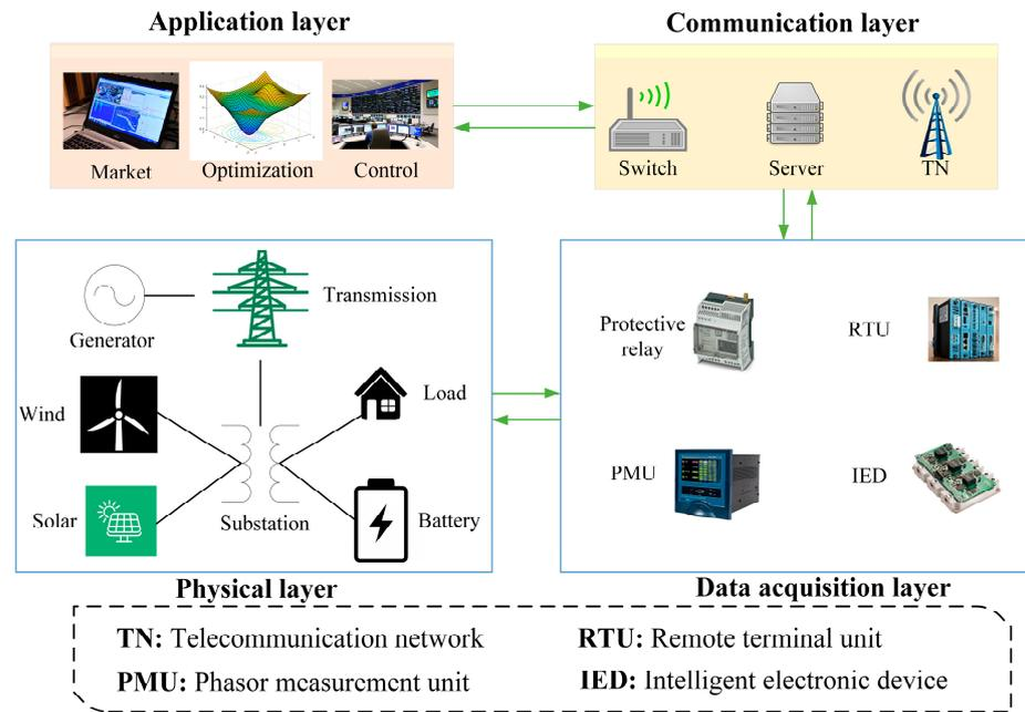
Figure 3. Physical and communication structure of the smart grid [46].
