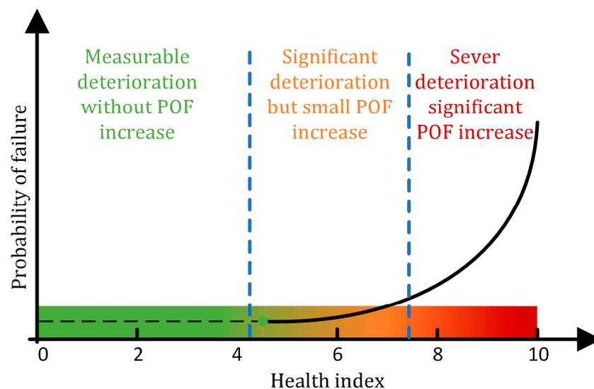
Figure 7. The increase in the probability of failure correlates with the rise in the health index [83].
