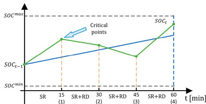
**Figure 11.** Reference trajectory of SOC (blue) and an example SOC curve (green) for a specific scenario during one operation hour.
