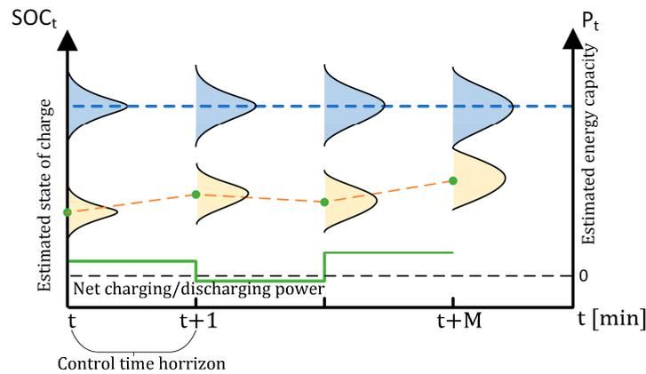
**Figure 10.** Estimated range of SOC (yellow) and energy capacity (blue) of ESS.
