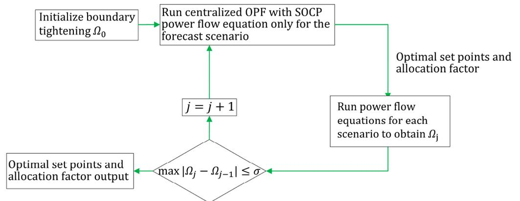
Figure 13. Boundary-tightening method.
