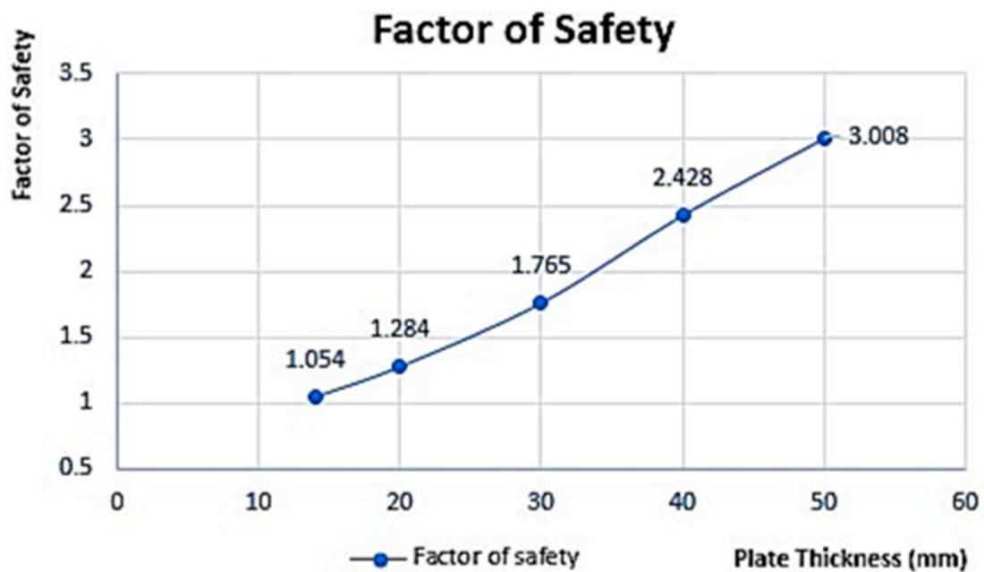
Figure 13. Factor of safety versus thickness.
