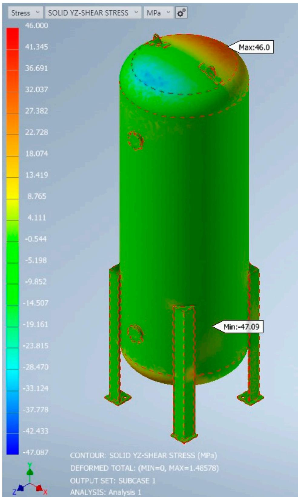
Figure 9. YZ-shear stress.
