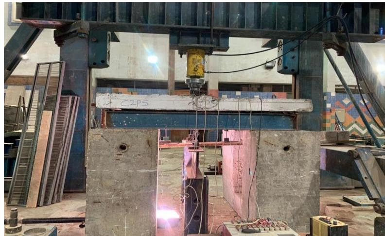
Figure 2. Test set-up for all tested specimens.
