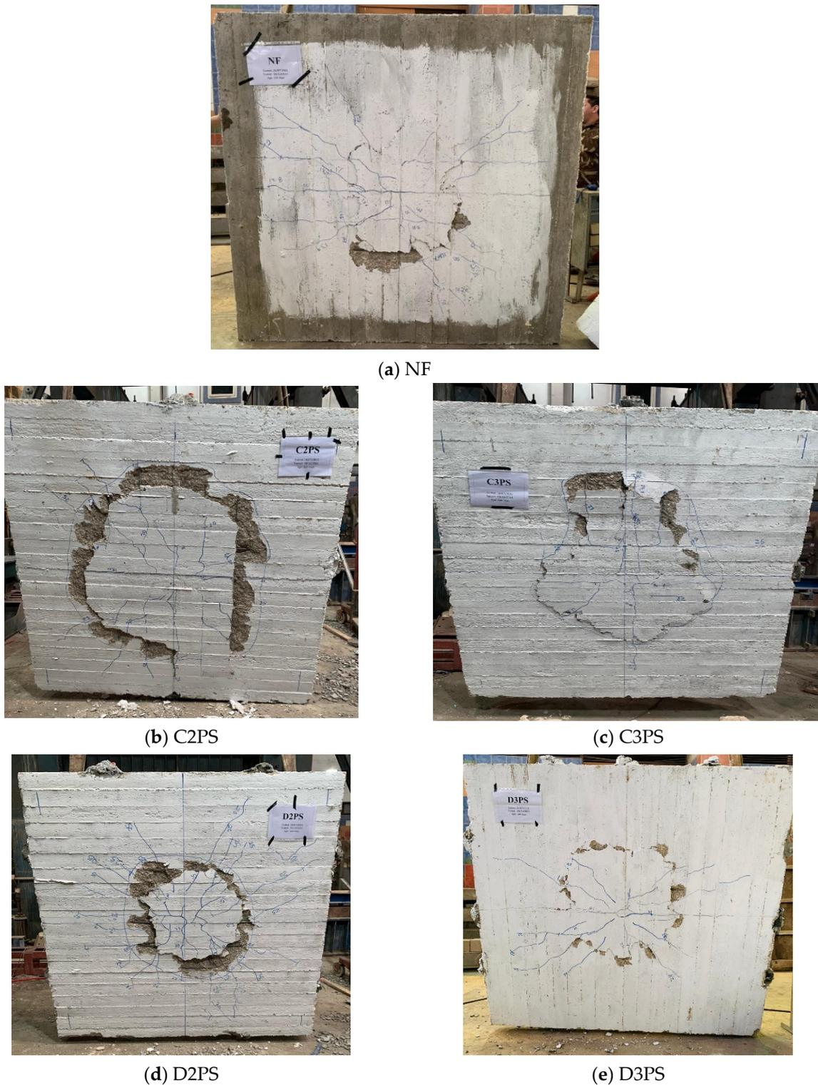
**Figure 5.** Failure mode of all tested specimens.
