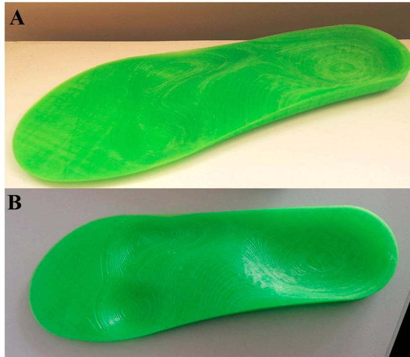
**Figure 4.** Right 3D-printed insole using thermoplastic polyether-polyurethane.
