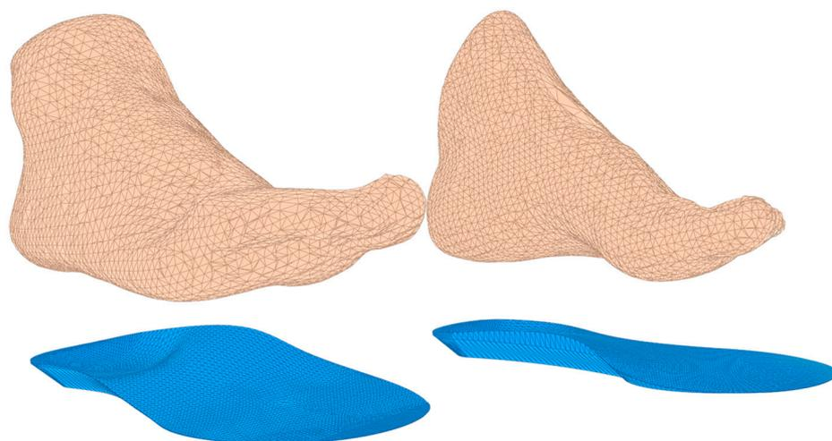
Figure A5. Scanned foot renders and insole design.
