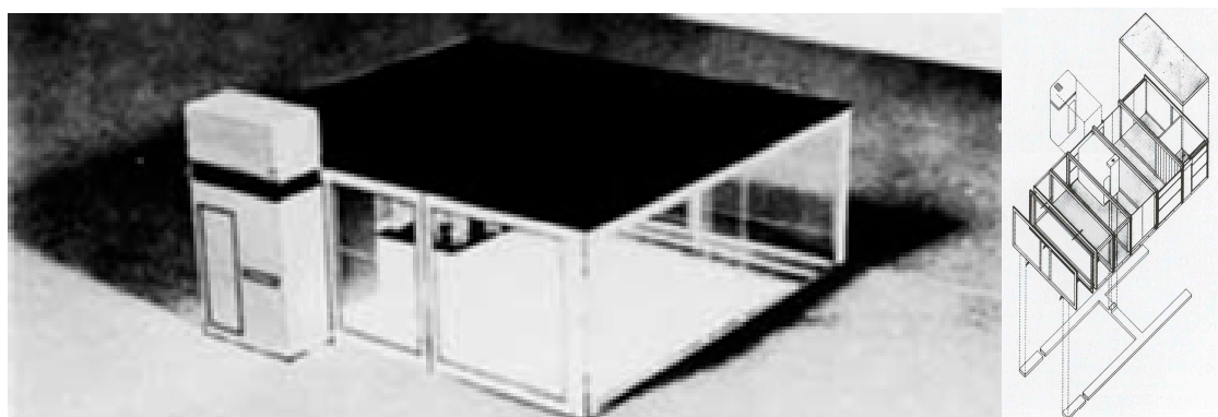
Figure 5. Steel Housing by Cedric Price, 1967: simple model, structure and connections [11].
